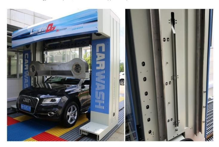
Contour-following air dryer with side air dryer
